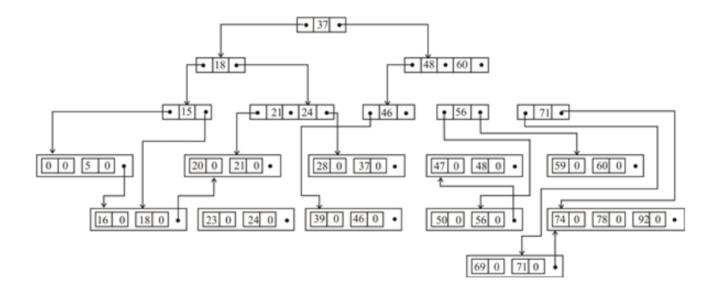
In the next step we may delete 18, it is in the right most entry in a leaf node and appears in an internal node of the  $B^+$ -tree. Now the leaf node is less than half full and combined with the next node.
